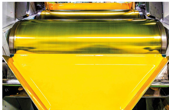
Ink production by three-roll mill
